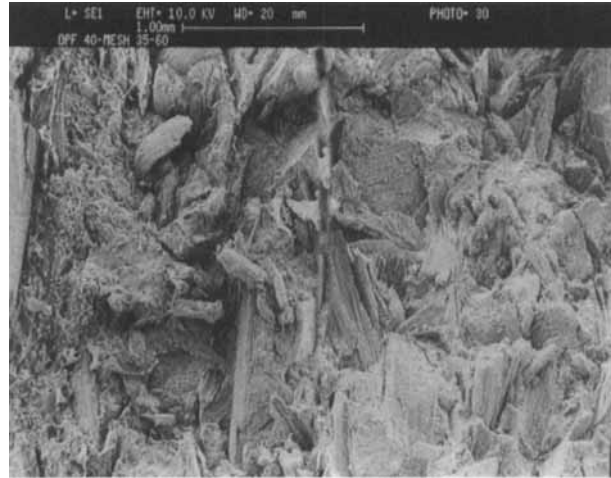
FIGURE 5 (A) –Scanning electron micrograph of tensile fracture surface of 40% OPF-PE composite. Magnification:35 X.
